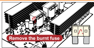
② Check one by one, find the blown fuse and pull it out.
