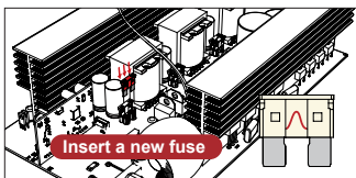
③ Replace a new fuse and insert it.
