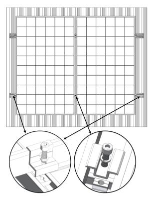
**Step 3.** Install the first solar panel and fasten it with the end clamps, and then insert the second solar panel and fasten it with the middle clamps and the end clamps.
