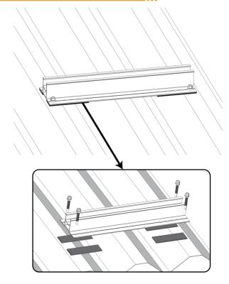
**Step 2.** Bond the rubber pads to the solar mounting rails, and then mount the rails to the roof with Screws.
